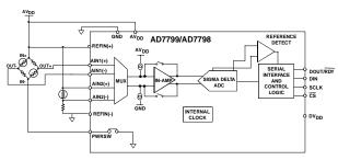
Figure 12. Basic Connection Diagram
