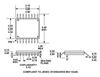
Figure 21. 16-Lead Thin Shrink Small Outline Package [TSSOP] (RU-16) Dimensions shown in millimeters
