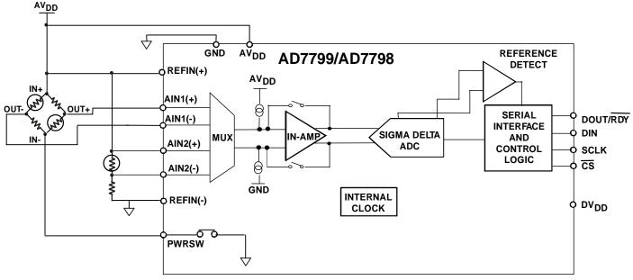
Figure 20. Weigh Scales Using the AD7798/AD7799
