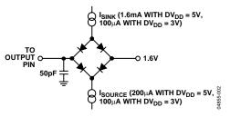
Figure 2. Load Circuit for Timing Characterization
