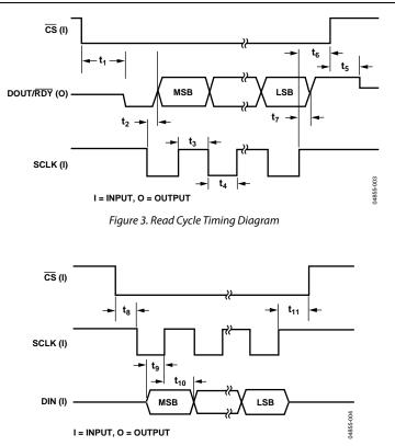
Figure 4. Write Cycle Timing Diagram
