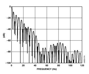
Figure 13. Filter Profile with Update Rate = 4.17 Hz
