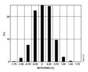
Figure 9. Excitation Current Matching (1 mA) at Ambient Temperature
