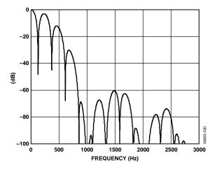
Figure 15. Filter Profile with Update Rate = 250 Hz
